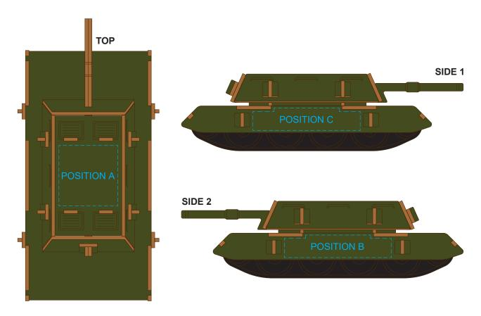
Up to a 2mm tolerance is expected for alignment of the printed artwork against the engraved lines. Slight inconsistencies are to be considered acceptable if the artwork is printed over an engraved line.
